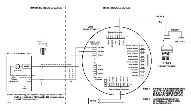
Figure 12—GT3000 Wired Directly to the UD10 Display Unit / UD10 Wired to PLC with 4-20 mA Isolated Sourcing Output
