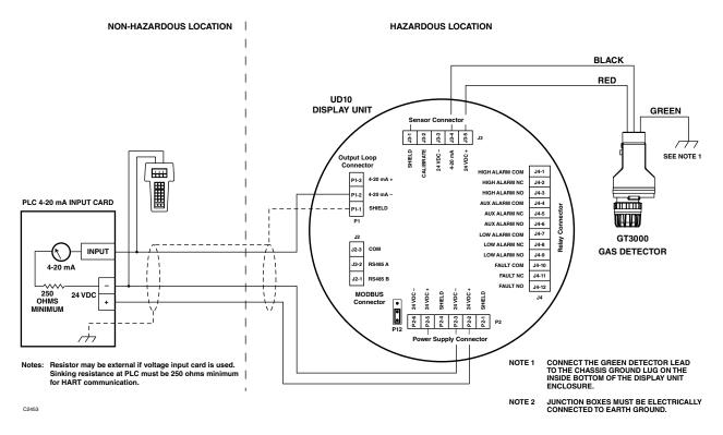
Figure 11—GT3000 Wired Directly to the UD10 Display Unit / UD10 Wired to PLC with 4-20 mA Non-Isolated Sourcing Output
