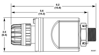
Figure 4—Dimensions of GT3000 Gas Detector in Inches (CM)
